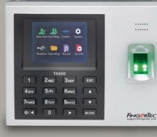
If you are looking for an affordable, reliable and simple biometrics time attendance clock, TA500 is your ultimate choice. It can contain up to 2000 fingerprint templates and 80,000 transaction logs in its flash memory at any given time. TA500 verifies fingerprint, password and it accepts embedment of card technology upon request. Equipped with the most commonly used IP communication method and USB flash disk, TA500 is the most powerful simple attendance system for your small and medium offices.
